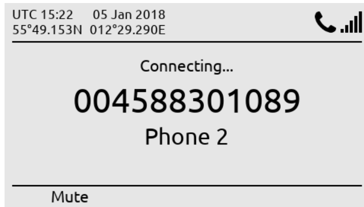
Figure 28: LT-3110 Control Unit – voice call connecting...
