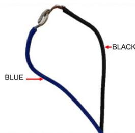
Figure 6: Blue and black wires joined together
