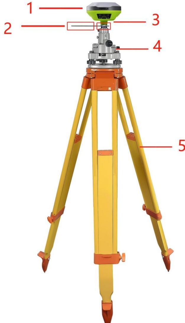
Figure 4.1 LUKA as a base - network mode
