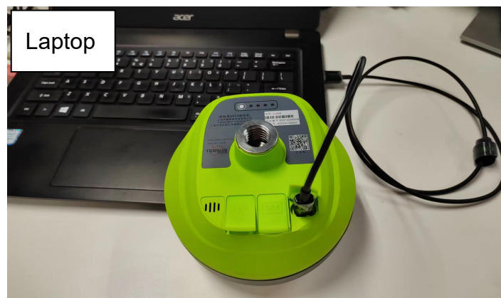
Figure 2.13 Connect LUKA to a computer
